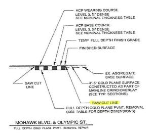
**Response:** This is an error. The edges of the cold plane pavement removal areas do not need to be sawcut.
